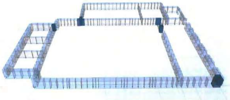
Figure 3.15: Regions where allowable bearing pressure is exceeded for 100%NBS loading.
